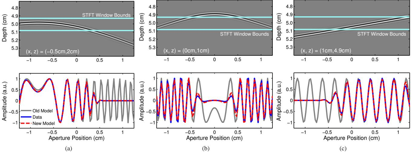
Fig. 1: Three examples are shown for the time-domain channel data and the corresponding aperture domain data after the STFT has been applied axially. The examples show several cases of  $x_n$ ,  $z_n$ , and  $\tau_n$  for a region of interest centered about 5 cm. Comparisons are made between the data, the new model and the old model in each of the bottom graphs.
