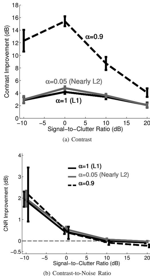
Fig. 10: The results of cluttered anechoic lesion simulations are shown as boxplots for several levels of signal-to-clutter ratio. Results are shown for several different sets of regularization parameters. The results mostly show that the ADMIRE images are better, but with very high or very low levels of signal-to-clutter ratio the improvement is not substantial. The largest improvement are seen from the images formed using  $\alpha = 0.9$  and  $\gamma = 0.5$
