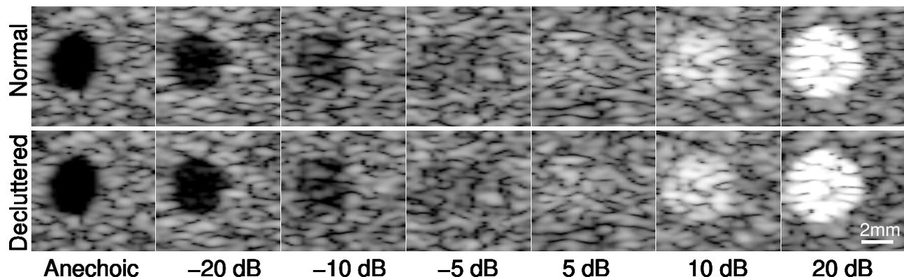
Fig. 7: 4 mm lesions are visualized using a 3 MHz F/2 imaging system. The contrast of the simulated phantoms goes from completely anechoic to +20 dB. For all cases there is little change between the decluttered and normal B-Mode data. The full summary of all the simulations is shown in Fig. 8, but the result is that the decluttering algorithm does not produce images with worse image metrics in the absence of clutter.
