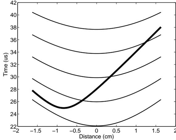
Fig. 2: When multipath scattering does occur the wavefront will extend across multiple dynamic receive delay profiles. This is demonstrated in the graph above with several receive delay profiles shown as thin lines, and a wavefront delay profile from modeled multipath scattering shown as a black line.
