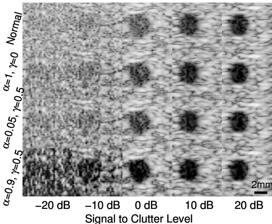
Fig. 9: 4 mm lesions are visualized using a 3MHz F/2 imaging system. The contrast of the simulated phantoms goes from completely anechoic to +20 dB. For all cases there is little change between the decluttered and normal B-Mode data. The full summary of all the simulations is shown in Fig. 10, but the result is that ADMIRE does not produce images with worse image metrics in the absence of clutter.
