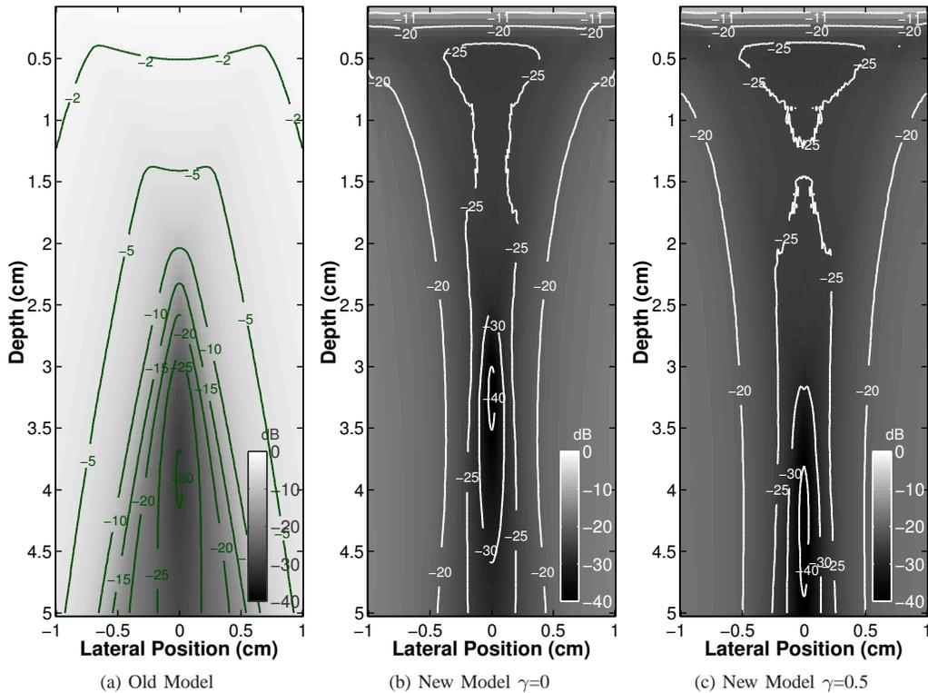
Fig. 4: Model error power is shown for the old model (a), the proposed model without additional modulation (b), and the new model with an additional modulation corresponding to  $\gamma = 0.5$  (c). The new model has distinctly lower model error compared to the old model. The new model has low error for both cases, but the case of the intentional receive modulation has slightly lower error.
