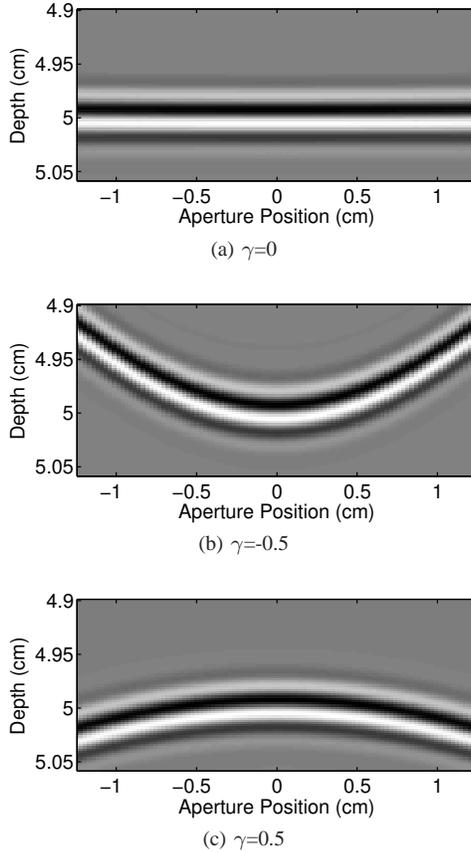
Fig. 3: Three examples are shown for different dynamic receive  $\gamma$  scales. When  $\gamma$  is negative the dynamic receive foci are shallower than normal so the wavefront becomes inverted, and when  $\gamma$  is positive the curvature from path-length differences is not entirely removed so some of the original curvature remains.
